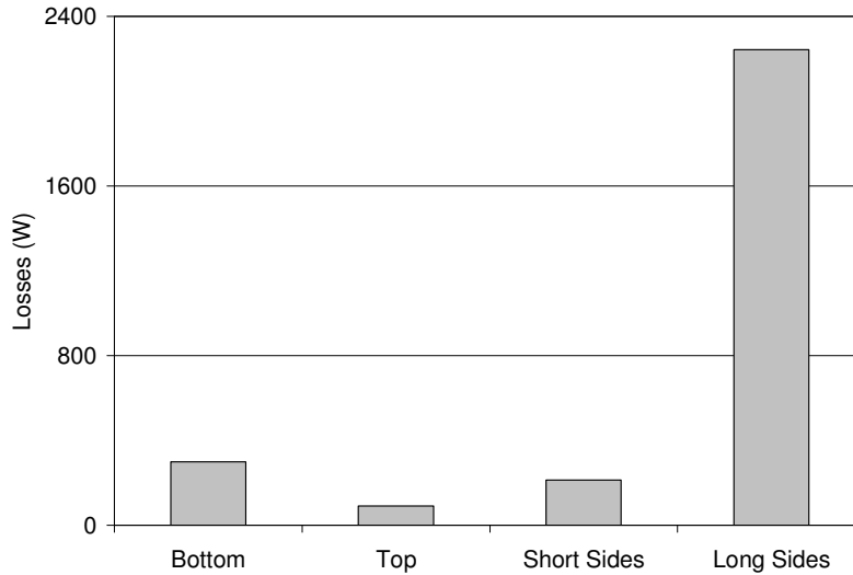
Fig. 2. Distribution of tank losses on its different walls for the original tank dimensions.
