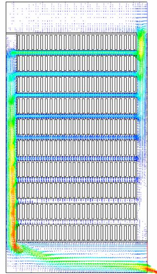
Figure 4 : Oil flow distribution with a group of discs
