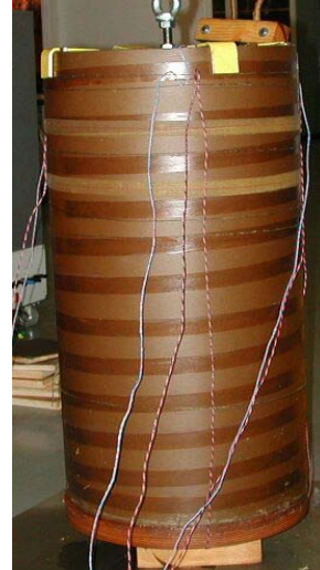
Fig. 1b: Winding equipped with sensors for local temperature measurements.
