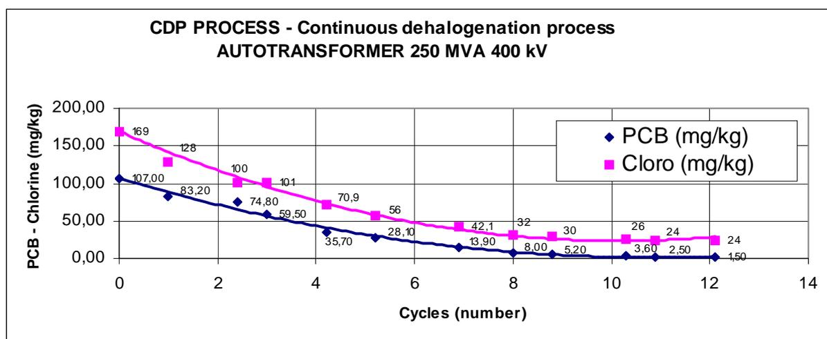
Figure 4 – Evolution of PCB and chlorine concentrations during dehalogenation process
