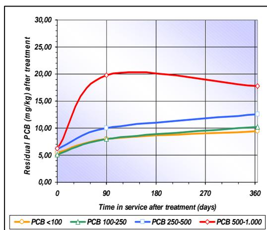
Figure 5 – Evolution of residual PCB concentration after one year of the treatment
