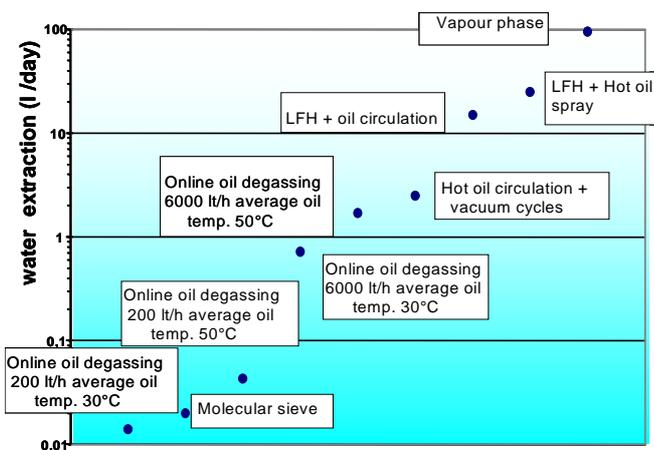
Fig. 5 : Drying velocity from 3% down to 1,5 % average humidity
