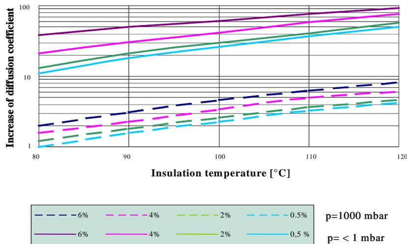
Fig. 2: Relative increase of the diffusion coefficient of a non-impregnated pressboard at different moisture levels, process pressure and temperatures [4] [6]
