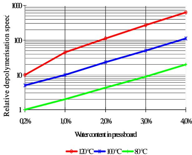
Fig. 1: Comparison of the relative depolymerisation velocity at different water content of a non oil-impregnated insulation paper [2] [6]
