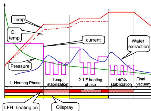
Fig. 4 : Process diagram of an LFH drying process with "hot oil spray"
