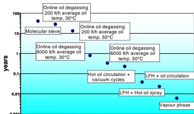
Fig. 6: Drying time to dry a 400 MVA transformer with 14 ton insulation from 3% down to 1,5 % average humidity
