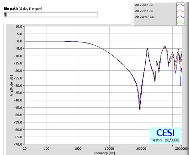
**Figure 4: Measurements carried out on the LV windings with the HV winding short-circuited**
