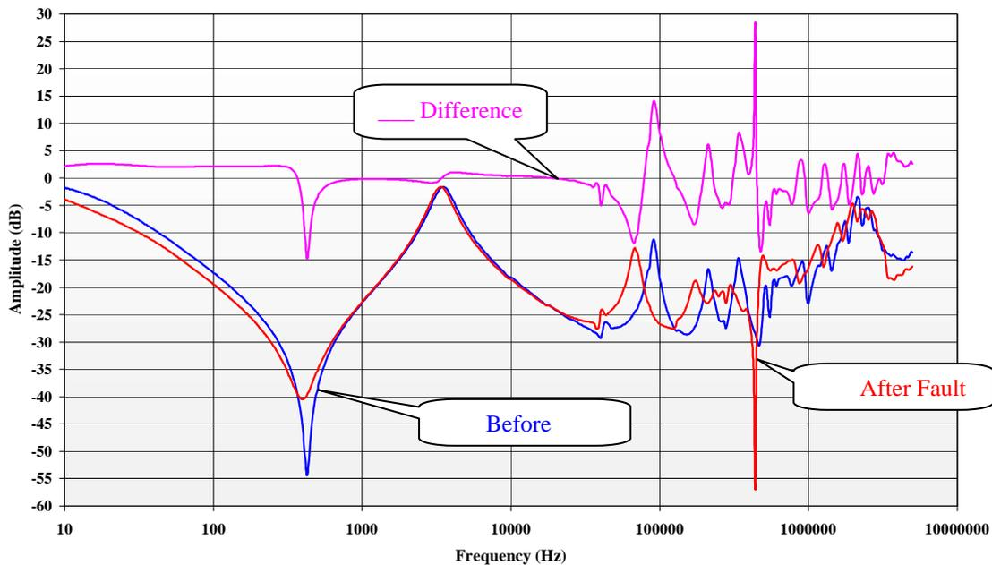
**Figure 8: Measurements carried out on the LV winding LV2 with the HV windings open; trace of difference is shown**
