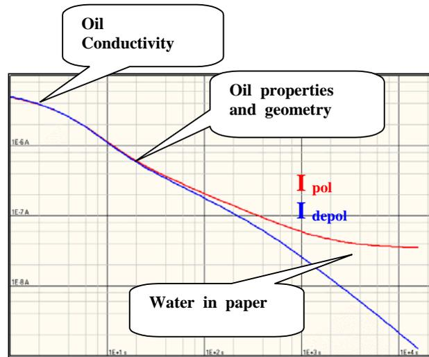
**Figure 12: Main influences on PDC curves in transformer oil-paper systems**
