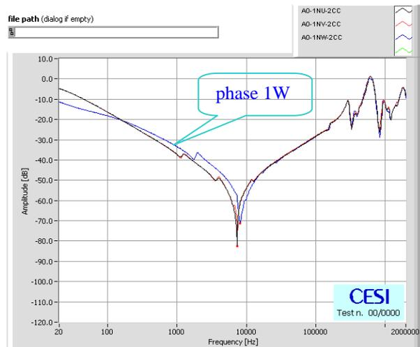
**Figure 2: Measurements carried out on the HV windings with the LV winding short-circuited**
