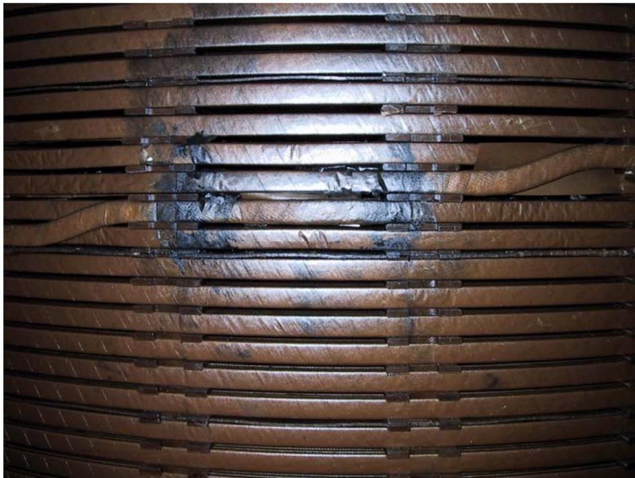
**Figure 5: Damage to the HV winding of phase W as seen after opening of the machine**
