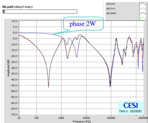
**Figure 3: Measurements carried out on the LV windings with the HV winding open and floating**
