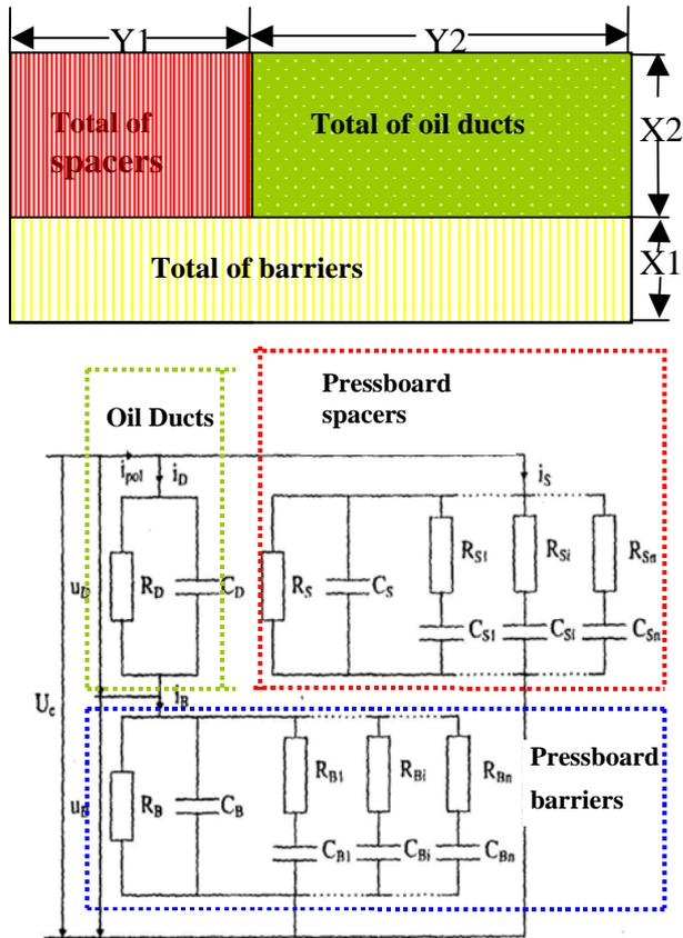
**Figure 11: Lumped insulation system and equivalent circuit of the main insulation of a power transformer**
