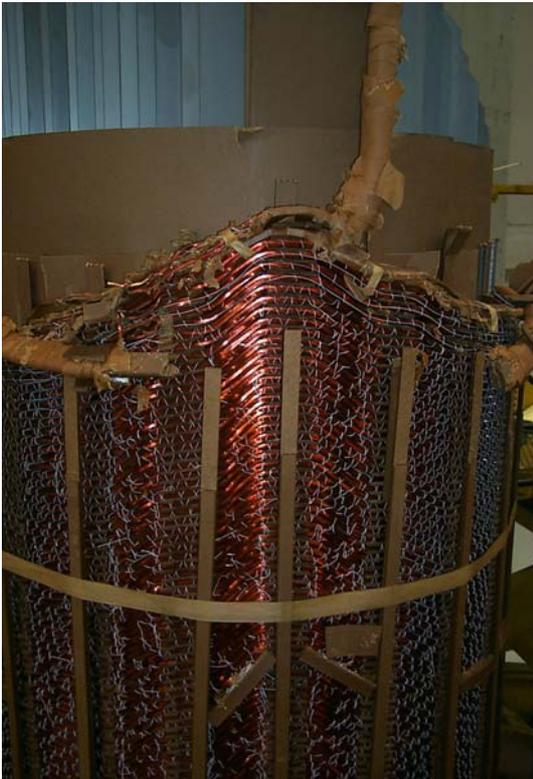
**Figure 9: Damage to the low voltage winding LV2 as seen after opening of the machine**
