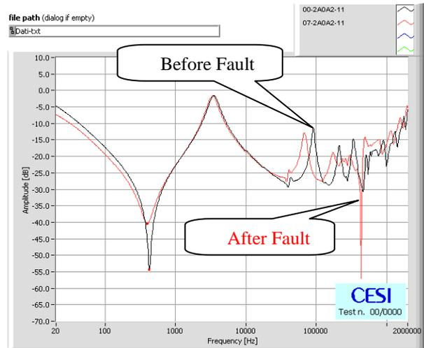
**Figure 7: Measurements carried out on the LV winding LV2 with the HV windings open**
