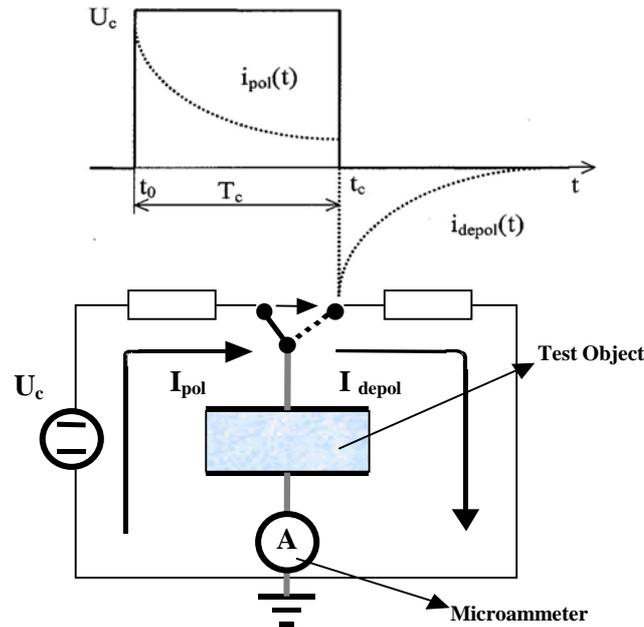
**Figure 10: The working principle and test circuit for the measurement of currents  $i_{pol}(t)$  e  $i_{depol}(t)$**
