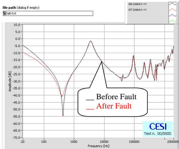
**Figure 6: Measurements carried out on the LV winding LV1 with the HV windings open**
