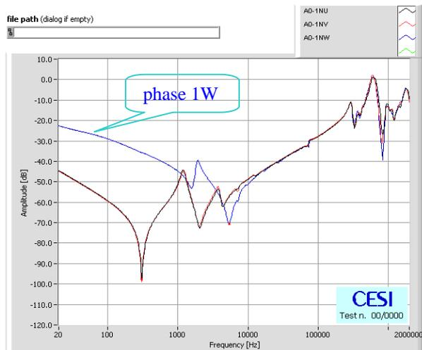
**Figure 1: Measurements carried out on the HV windings with the LV winding open and floating**
