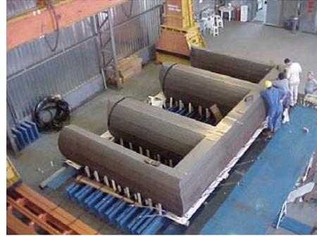
Figure 7 – Core Repair (assembled core mass: 173tons)
