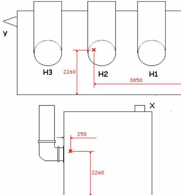
Figure 5 – PD Location Acoustic Sensors and Triangulation Method
