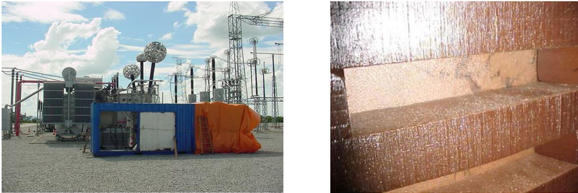
Figure 4 – Transformer (300MVA, 550kV) under HV On-site Testing and PD Location
