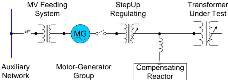
Figure 2 – Test Setup Single-Line Diagram
